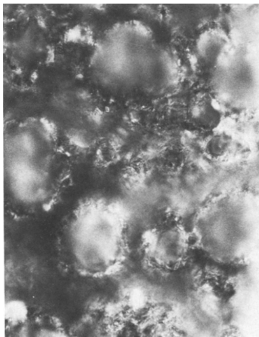
Fig. 9. The structure of a typical anode surface in the wake of oscillatory current behaviour: (a) overall electrode surface; (b) micrograph of the oxide deposit (upper left portion); (c) micrograph of the dissolution region (lower right portion).
